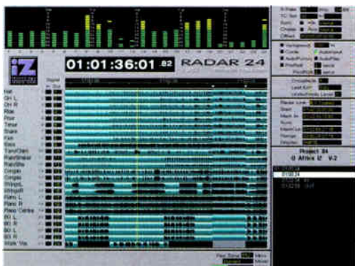
RADAR main screen shows meters, status and waveforms.
