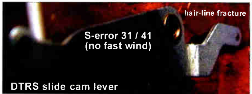
Figure 3 A hairline fracture of the slide cam lever can cause fast wind failure (S-error 31/41).
