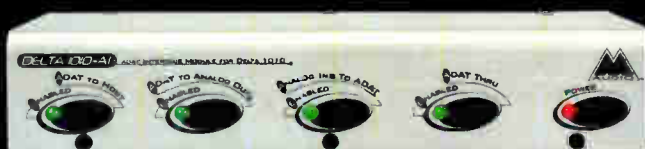
DELTA 1010-AI - ADAT interface add-on for DELTA 1010
