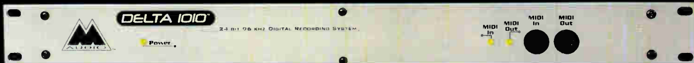
DELTA 1010 - 10 in/ 10 out PCI digital recording system.
