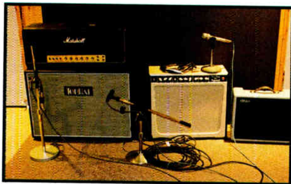
Froom and Paterno like to record guitars through many different-sounding, mostly small amps. The mics are an SM57 and a KM86.
