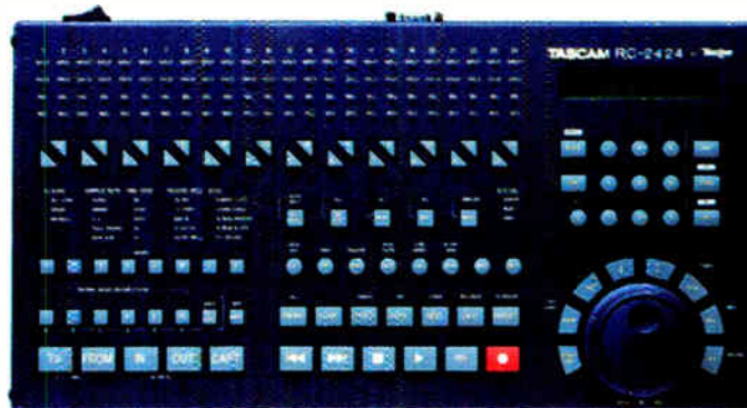
The RC-2424 remote duplicates all front panel functions.
