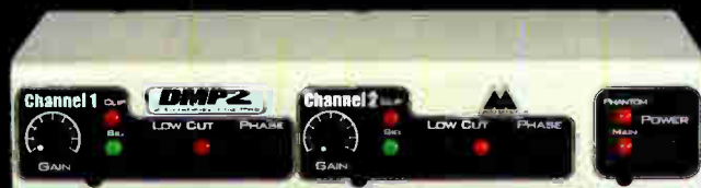
DMP2 - 2 channel mic preamp direct box.
