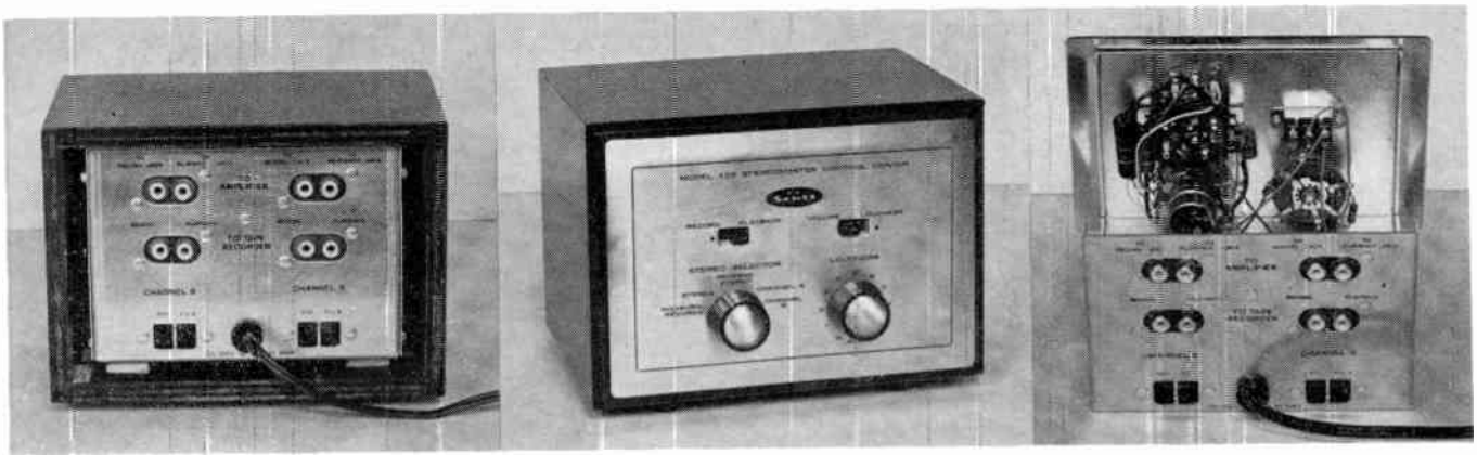
Fig. 1. Rear, front, and inside views of a master switching and volume control unit for stereo systems using separate preamps and amplifiers
