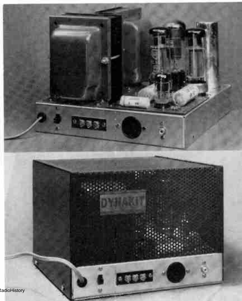
Fig. 6. Dynakit completed except for cover and bottom plate. Fig. 7. Only the terminals and the power switch are exposed when the cover is in place
