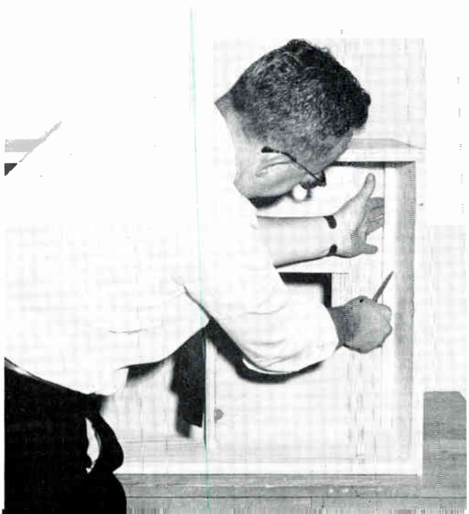
Fig. 2. Front view, locating the speaker board brace under the shelf
