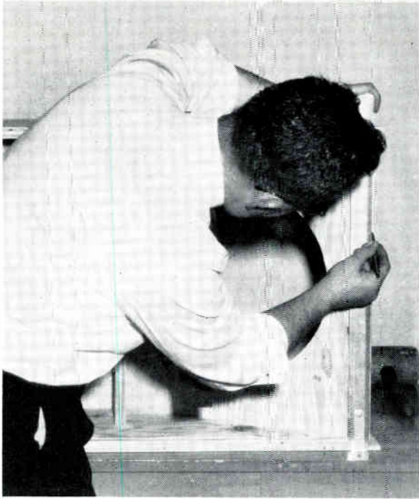
Fig. 1. Front view, fitting the speaker-mounting board at the bottom
