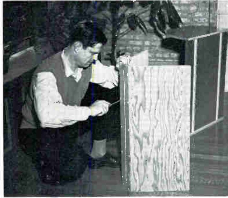
11. The finished corner enclosure was assembled in about 40 minutes. No fuss, no muss, no dust! All the exposed wood came sanded, ready for shellac or stain. Speakers can be changed later, or a second 12-in. speaker can be added by removing the disc from the upper opening.
