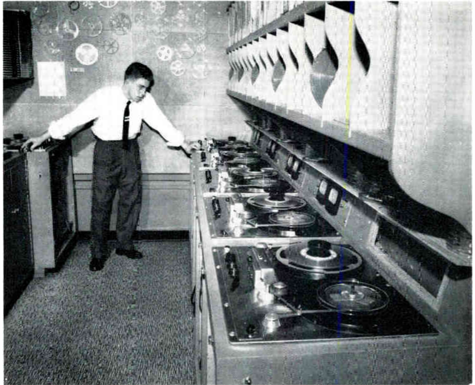
Fig. 3. Engineer Robert Kelly, of Audio-Video, operates five special Ampex recorders, making tape copies from a master tape on the playback machine at the left. Using two record heads, these machines copy two tracks simultaneously at four times normal playing speed, and operate at frequencies up to 60,000 cycles
