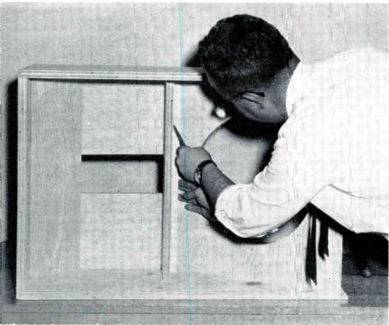
Fig. 2. Front view, locating the speaker board brace under the shelf
