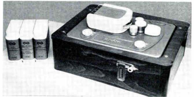
Fig. 2. Pickup at right can be set by knob on front of cabinet, follows grooves on the belt. Playing time is 2 to 8 hours, depending on the speed and length of the belt
