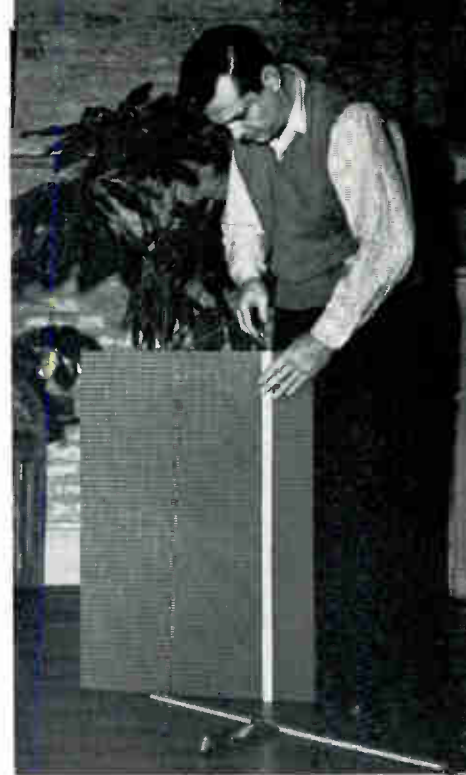
3. Left: A disc is furnished to cover the upper opening if only one speaker is to be used. Bolts and nuts are positioned according to RETMA standards.
