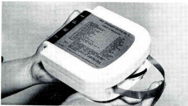
Fig. 1. This magazine holds a continuous plastic belt, up to 600 ft. long, driven from beneath
