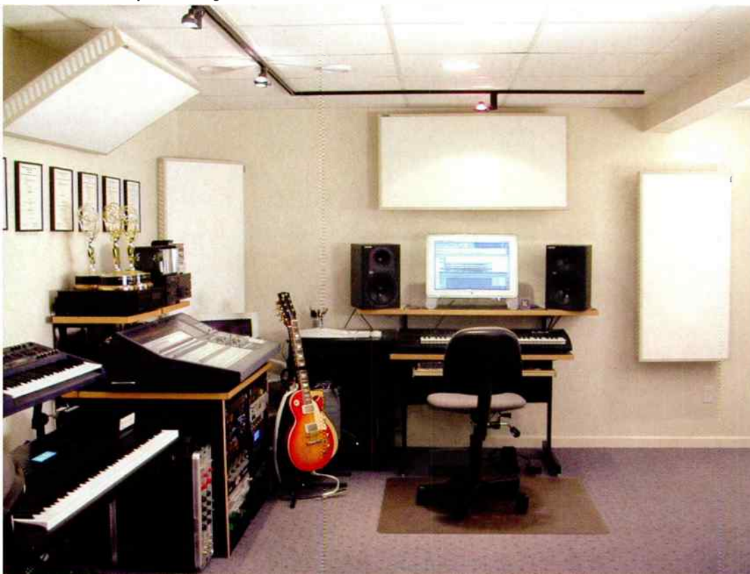
Fig. 1: Absorption panels, such as the Realtraps Minitraps (pictured), can be placed strategically to make an architecturally disadvantaged studio shine with sound.
