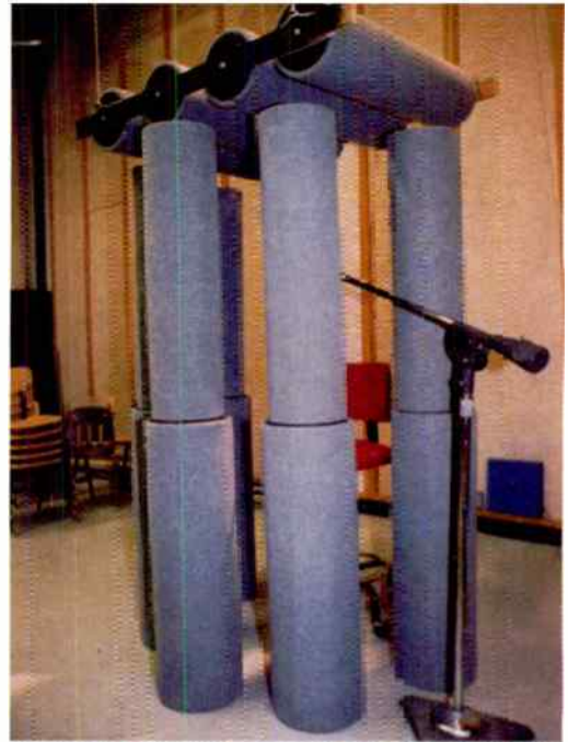
Fig. 3: This early QSF setup (circa 1987) uses an overhead QSF "cloud" to help hold in upward energy.
