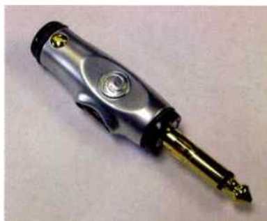
Fig. 1: Note the recessed "Circuit Breaker" switch toward the left side of this 1/4" plug.
