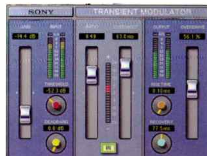
Fig. 3: Sony's Transient Modulator takes the sting out of excessively spiky attacks.
