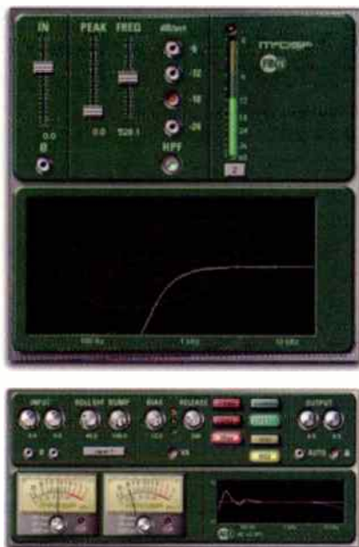
Fig. 2: A high-pass filter passes frequencies above a particular cutoff frequency, which can help clean up muddy bass in your mix.
