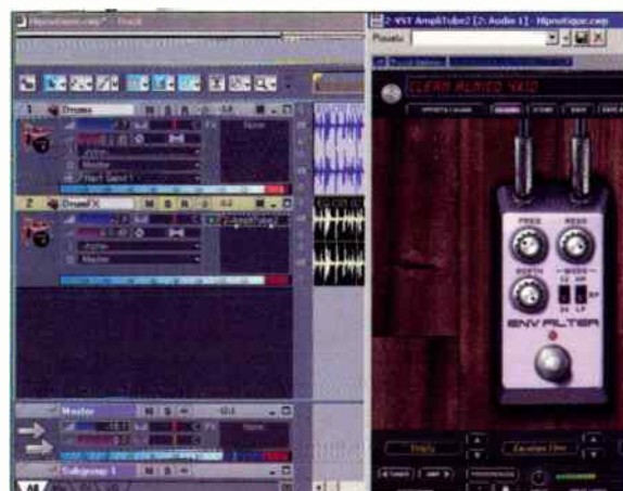
Fig. 2: Envelope filter effects work really well with drums. Here, a drum track has been copied, with the effect added to the copy only.
