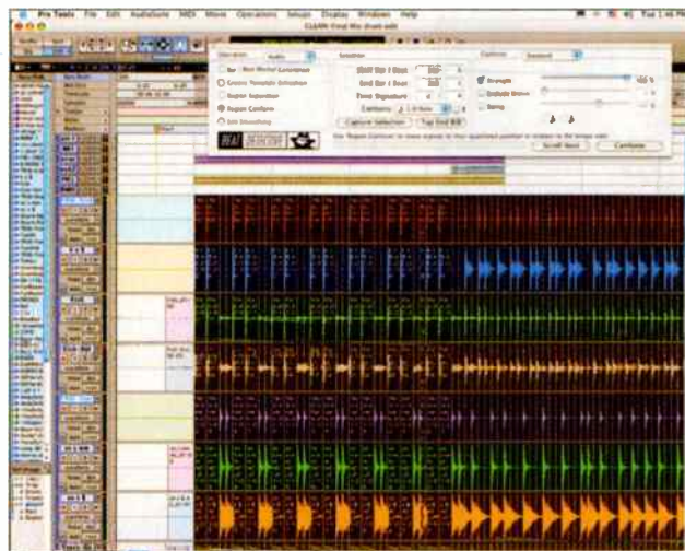
Fig. 2. Usually it is best to conform the selection to 100% strength, which will place each piece of cut audio onto the Pro Tools grid. Because this will not necessarily give a desired feel, move each piece to where your ears want it to be.
