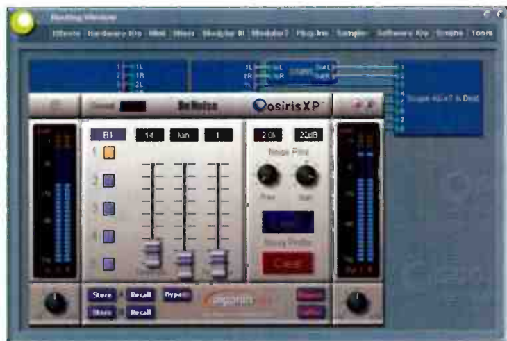
Fig. 3: The OsirisXP noise reduction module is being called up by itself; the background Scope routing window shows it patched into the system.
