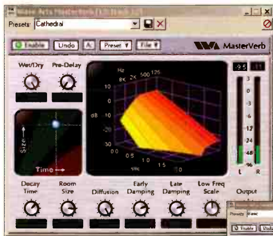
NOTE MASTERVERB’S 3-D DISPLAY, WHICH PROVIDES A VISUAL REPRESENTATION OF TIME AND FREQUENCY RESPONSE.
