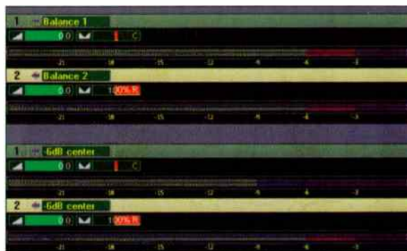
Fig. 4: Note the difference in the center channel signal level between the Balance and -6dB center options.
