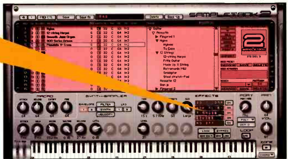
SAMPLETANK 2 HAS AN OBVIOUS, FRIENDLY INTERFACE. THE UPPER LEFT SHOWS A MIXER WHERE YOU CAN ASSIGN INSTRUMENTS TO THE 16 MIDI CHANNELS; THE BROWSER IS IN THE UPPER RIGHT. BELOW THESE ARE THE EDITABLE PARAMETERS, AND A VIRTUAL KEYBOARD.
