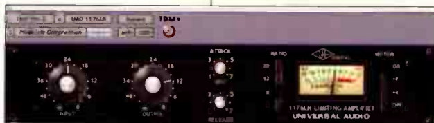
THE 1176LN PLUG-IN IS FEATURE-ACCURATE WITH THE HARDWARE VERSION. IT'S DSP-HUNGRY, BUT FAITHFULLY RECREATES THE SOUND AND RESPONSE OF THE ORIGINAL.
