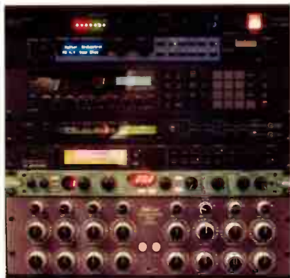
Processors at Ironworks include a Lexicon PCM90, Yamaha REV7 and SPX90II, TC Electronic D-Two, and a Line 6 Echo Pro.
