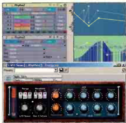
Fig. 3: The audio track contains two envelopes for parameter control; the MIDI track contains two more, as well as a controller curve from a MIDI fader box's output.
