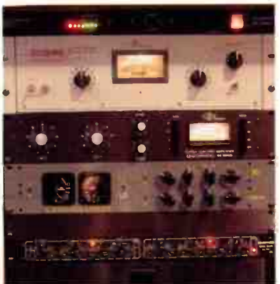
Dynamics processors in regular use at Ironworks include a Universal Audio LA-2A and 1176LN, a Chandler Ltd. TG1, and a Drawmer DS201.
