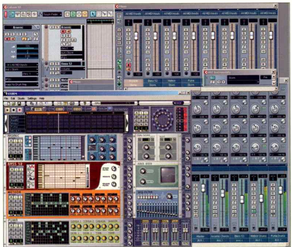
The upper left shows the MIDI tracks driving various Storm instruments. Moving clockwise, note the corresponding faders in the MIDI mixer, VST Instrument window where Storm is called up, VST Audio mixer (note the five audio channels containing Storm's audio), and finally, the complete Storm instrument.
