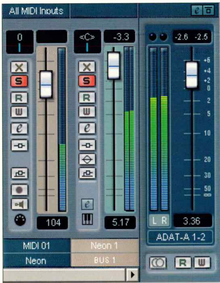
Fig. 1. The VST Instrument and MIDI Track driving it have both been soloed; the audio is being checked for distortion prior to bouncing.
