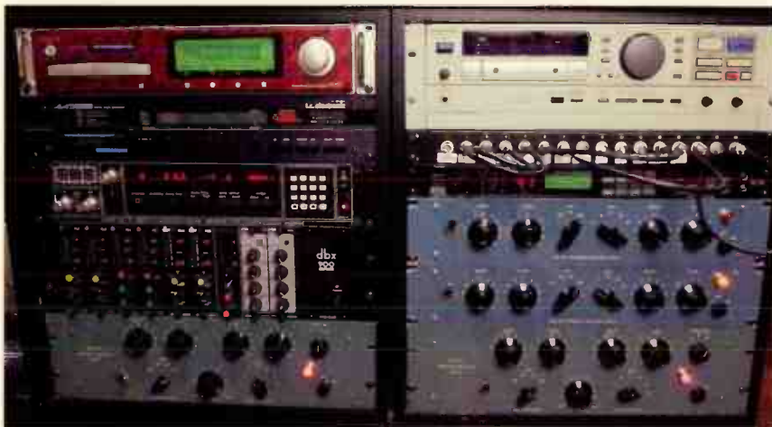
The racks at Michael Bacon Studios comprise a variety of tube, analog, and digital processing gear. Shown here are (left side) Sony DRE 777, TC Electronic M5000, AMS RMX-16, dbx 900 rack, Pultec EQH 2; (right) Panasonic SV3700 DAT, patch panel, SPX 1000, two Pultec EQP 1-A, Pultec EQH 2.
