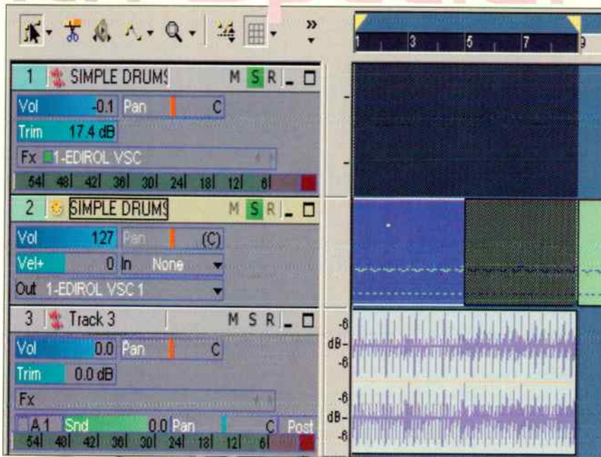
Fig. 2. Measures 1-9 have been selected for bouncing; Track 1 holds the instrument (Editor's VSC), Track 2 the MIDI data that drives it, and Track 3 is the resulting audio mixdown.
