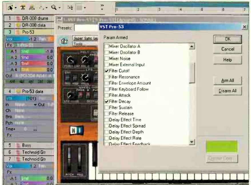
Fig. 2: Right-clicking on the Pro-53 instrument name in Track 3 brings up a list of automatable parameters.
