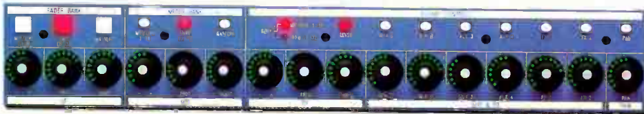
...OR A SET OF ROTARY LEVEL CONTROLS FOR THE TAPE RETURNS.
