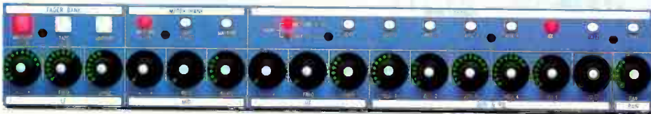
...OR A ROW OF 16 AUXES OR FX SENDS FOR THE 16 FADERS BELOW THE E STRIP...
