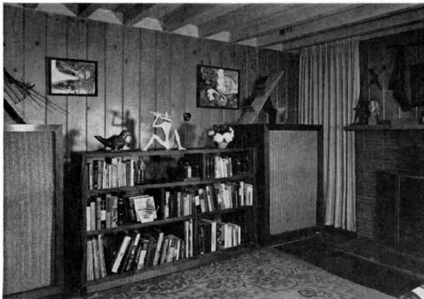
The "fronts" of speaker systems shown here are really enclosure backs. Woofers face walls, while dummy grille cloth gives the illusion of bass speakers facing into the room. ("... gives me just the right dispersion of sound," says Mavity.) Exposed mid-range horns and ribbon tweeters are placed at an angle chosen by our audiofan as the best ones after many hours of comparison.
