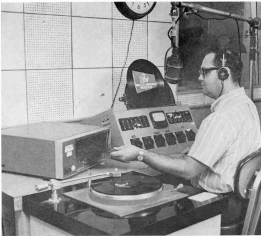
A broadcast station engineer (above) uses a magnetic mat for on-the-air playback of commercial messages. He can also record commercial material directly on mats if he wishes. The machine's drive system (left) includes a 7½ pound cast iron turntable which rotates at 12 rpm while a magnetic head mounted on a carrier tracks in a straight line across the circular mat as it rotates.
