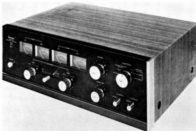
Sansui/quad synthesizer is a preamp-type unit, taking two-channel sources and producing four channels for direct feed to power amplifiers.
