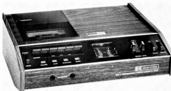
Harman-Kardon CAD 5 is one of several new cassette machines to incorporate Dolby "B" circuits.
