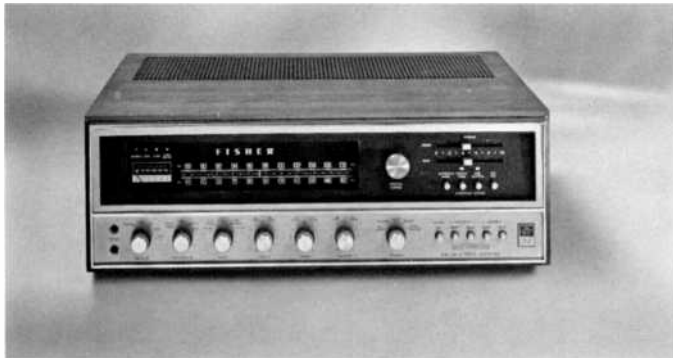
Fisher 701 quad receiver had conventional stereo FM/AM and amplifier plus two more amplifier channels for surround sound. Unit will also synthesize quad from existing two-channel program sources.
