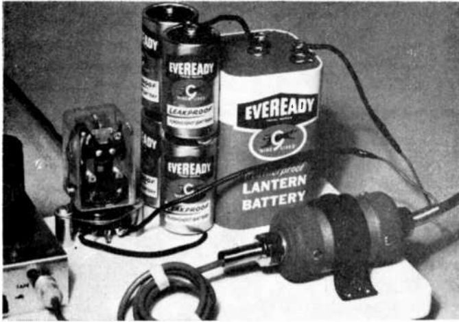
Fig. 8. Notice the extra batteries added in series/parallel to the lantern battery hookup. Although this relay is rated at six volts, a number of variables (such as going through two hundred feet of fine cable wire) makes it necessary to build up the voltage to nine volts or so for best and consistent results with the relay.
