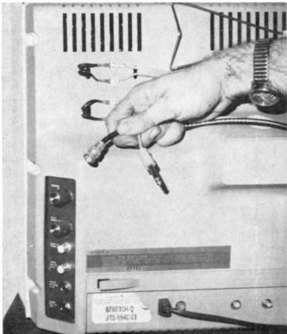
Connections on the rear of modified Motorola TV set supplied by Ampex are inputs and outputs for both video and audio. Top switch selects normal TV entertainment function or VTR function. Second switch selects matching line impedance for different kinds of connecting cables.
