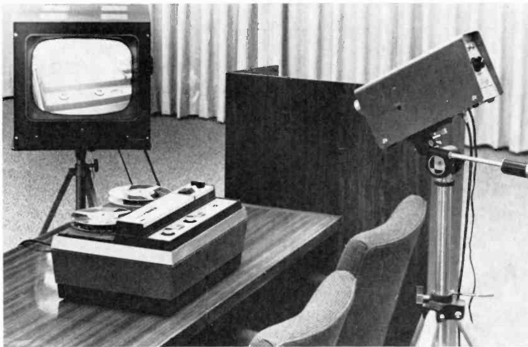
Designed as a training device for education, business, industry and the military, this new Wollensak VTR-150 video tape recorder from 3M Company records and plays back television signals, "live" programs recorded with an accessory camera, or pre-recorded tapes prepared on other VTR-150's.
