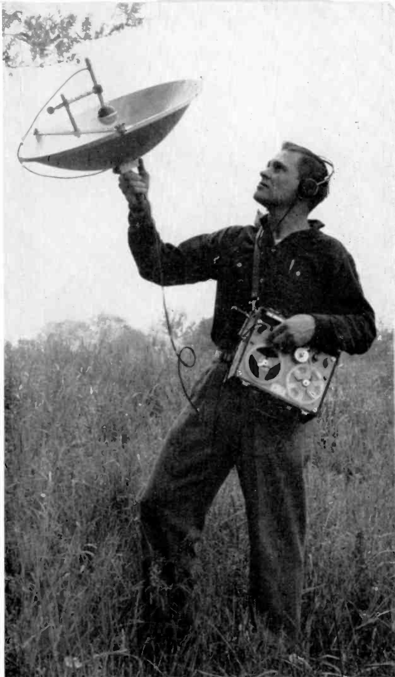
The author demonstrating the use of an aluminum parabolic reflector with the Magnemite Portable to record cicadas and other treetop singing insects.
