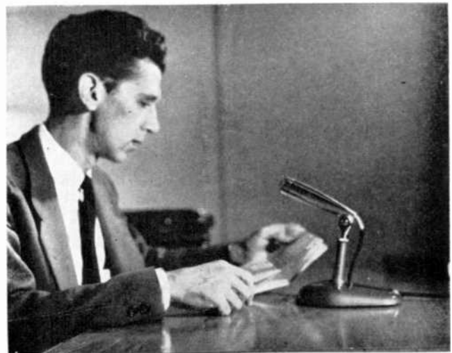
The desk stand makes it easy for commentators or those dictating letters to do their job. A hand held mike set on the table is always in danger of being knocked over, spoiling the recording.
