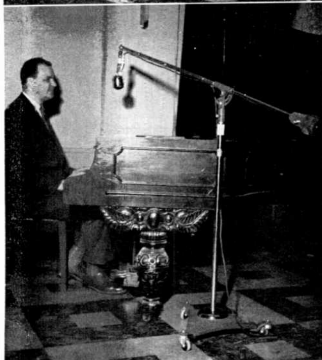
Top: For speakers who turn from side to side as they talk a twin mike setup is the best. As the volume falls off on one mike it picks up on the other. Such units as shown can be made up of mike stand accessories stocked by most radio parts houses. Lower: a boom mike stand should be used on a vocalist-piano pickup to keep the stand out of the way of the player's hands.
