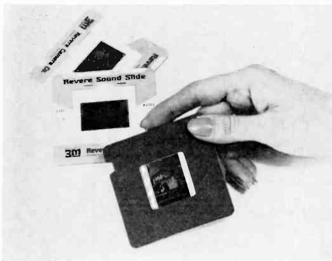
The new Reverse Sound Slide Projector may be the forerunner of a new type projector. It has the sound right on the slide mount and each mount will hold up to 20 seconds of recorded sound. Projector both records and plays back and slide changes are automatic. The recording head moves in a spiral path around the mount which is coated with magnetic material.
