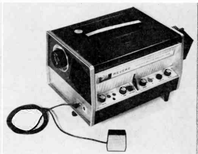
The new Reverse Sound Slide Projector may be the forerunner of a new type projector. It has the sound right on the slide mount and each mount will hold up to 20 seconds of recorded sound. Projector both records and plays back and slide changes are automatic. The recording head moves in a spiral path around the mount which is coated with magnetic material.
