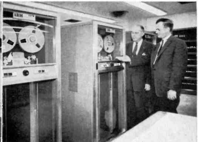
Left: Tape recorders are widely used in testing laboratories to achieve product improvement, especially in the automobile industry. Here noise level tests are run and recorded on tape for scientific comparisons between various muffler designs for industrial engines. Right: Tape handling units for an IBM electronic computer serve as versatile "filing cabinets" which store millions of bits of data, yet produce it upon command in a matter of seconds. Future developments will reduce size of units and increase storage capacity.
