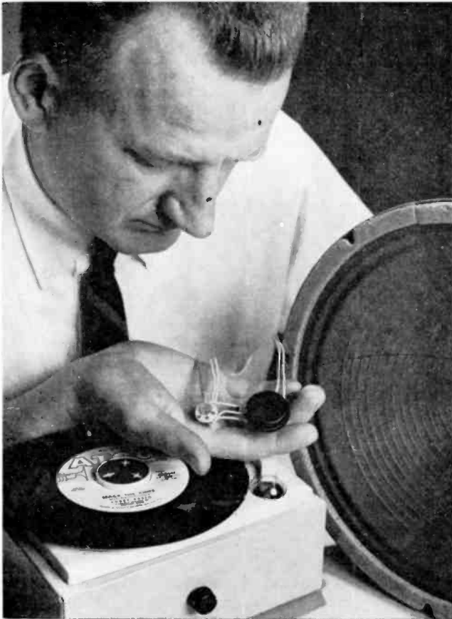
Above: an example of micro-miniaturization is this Westinghouse developed molecular electronic function block being used as an audio amplifier in a conventional system. Frequency range is 0 to 20,000 cycles and output is 5 watts. Amplifier itself (at right in black mounting) is tiny device whose volume is .001 cubic inch. Device at left is molecular electronic preamp.
