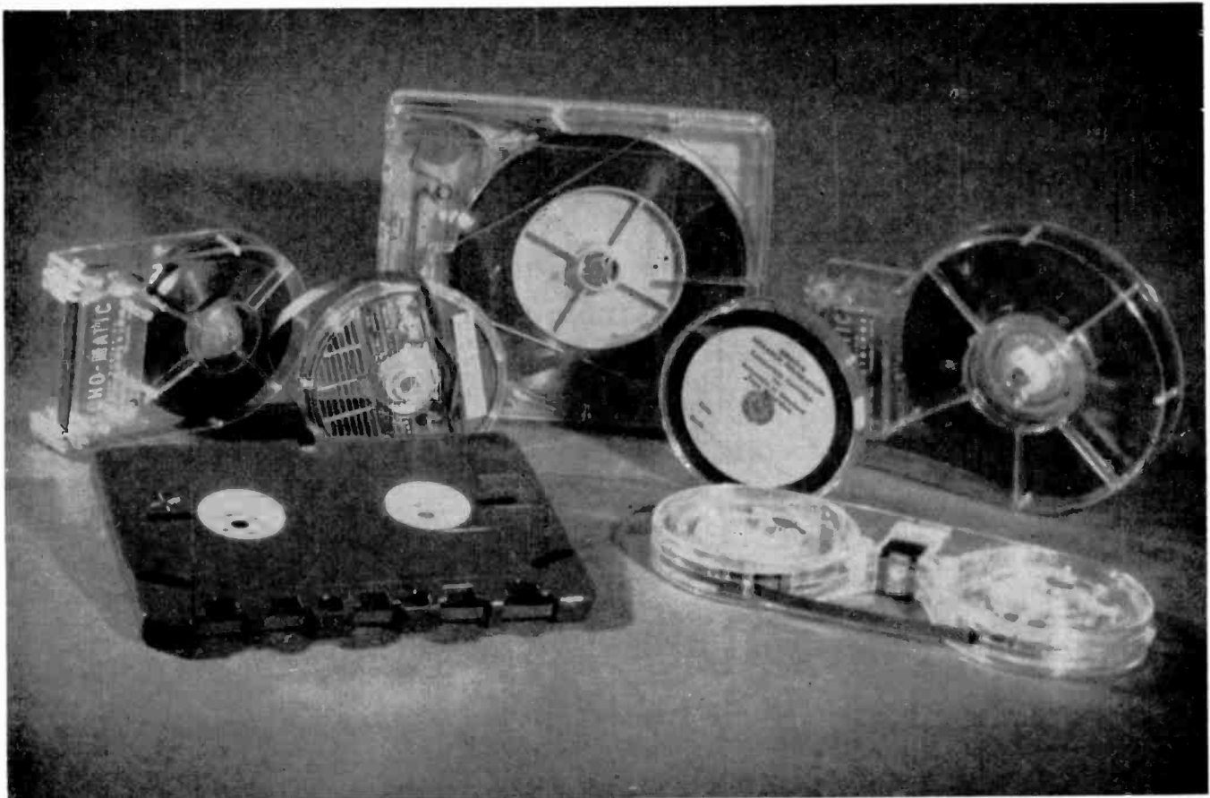
Cartridge developments over the years. Rear left and right is the Cousino continuous loop repeating cartridge in small and large sizes. In center is Fidelipac cartridge developed by George Eash in 1956. Circular cartridges are: left, Cousino Audio Vendor for use on standard machines and, right, Armour Foundation spool. At left foreground is RCA type cartridge and at right the cartridge used on Norelco dictating machines. Not shown is the new 3M cartridge shown on next page.
