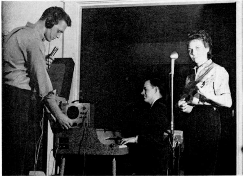
Output of the Wurlitzer Piano is fed directly to the mixer making the pickup, independent of room echo or noise. Any electrically amplified instrument can be so handled.
