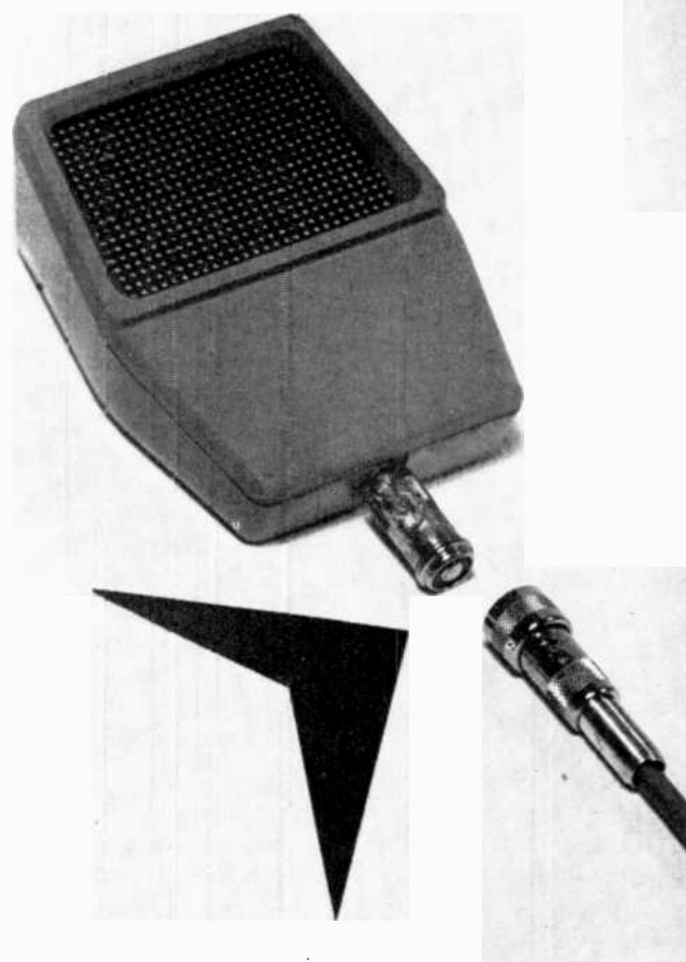
Fig. 10: Work cautiously when fastening the male mini-connector to the one-inch-long cable coming from the mike. Strip off the insulation, bring the shielding to the outside of the connector, then solder both it and the inner connector carefully, using a minimum of heat. Now test the mike on your recorder before proceeding.
