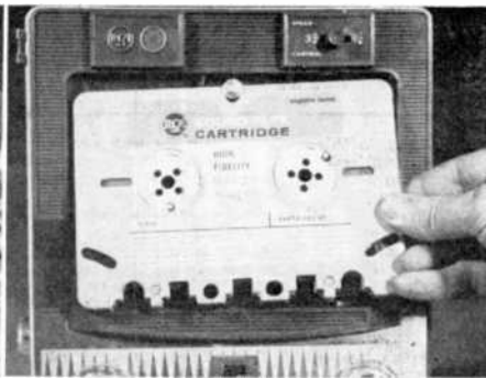
Left: inputs and outputs are grouped on the side of the case. From left to right: speaker switch, output, input, mike socket and on-off volume knob. Right: cartridge slips in place on top of case centering slot over the pin in the rear of the cartridge well.
