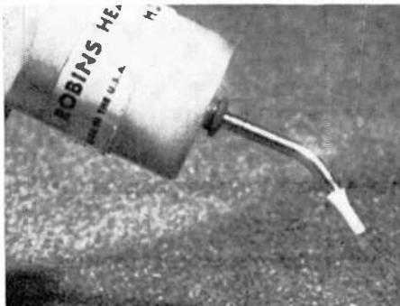
The shaft of the demagnetizer is of small diameter and this coupled with the angled bend makes it easy to reach the heads.
