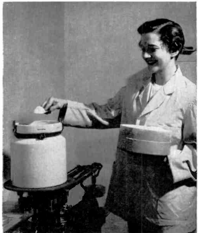
Ingredients such as wetting agents, anti-bloom compounds and binders are very carefully weighed and measured to insure a uniform coating for every batch of tape.
