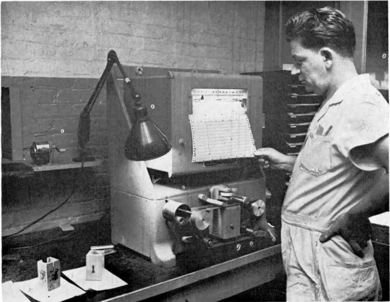
Samples of acetate film manufactured by Celanese Plastics Company at Newark New Jersey, are constantly tested on this automatic gauge recorder. The Celanese manufacturing process provides a film of exceptionally uniform gauge, with a tolerance of .00003 of an inch, being maintained. Any variation in the thickness of the film has an effect on the final oxide coating. The tolerance is only one hundredth the thickness of a human hair.
