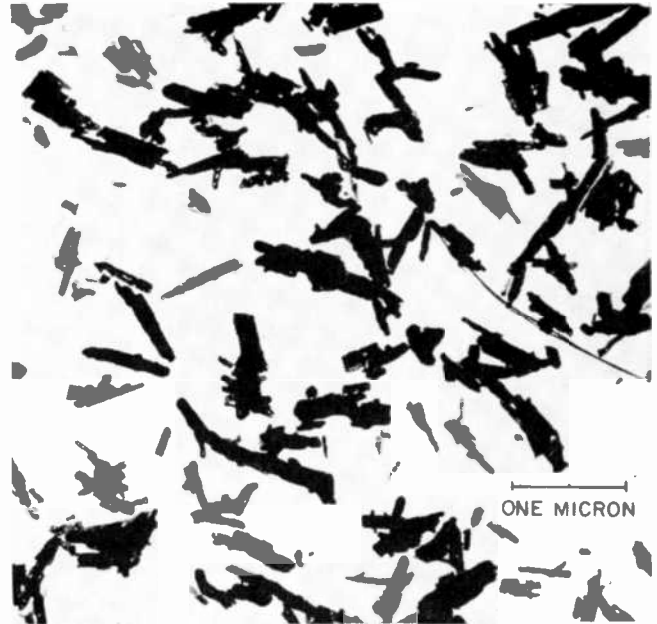
Left: the basic ingredient of magnetic tape's coating is iron oxide, a very carefully manufactured ingredient held to close tolerances. Photo courtesy Minnesota Mining and Mfg. Co. Above: a photo made through an electron microscope showing the needlelike particles of acicular iron oxide. Magnification is 35,000 times. Courtesy C. K. Williams Company.
