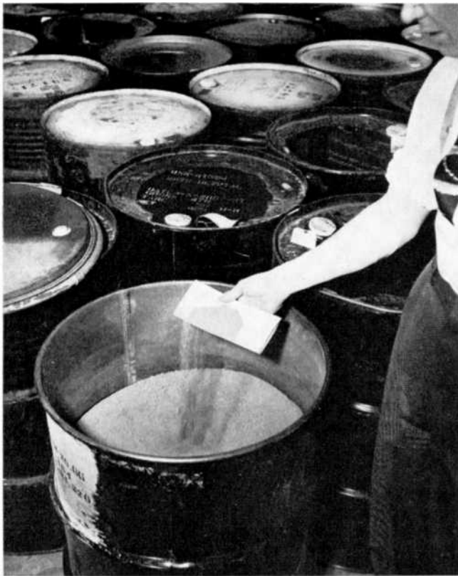
Left: the basic ingredient of magnetic tape's coating is iron oxide, a very carefully manufactured ingredient held to close tolerances. Photo courtesy Minnesota Mining and Mfg. Co. Above: a photo made through an electron microscope showing the needlelike particles of acicular iron oxide. Magnification is 35,000 times. Courtesy C. K. Williams Company.
