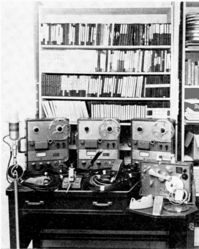
Foreground: part of the tape recording equipment used by Creative Associates, the machine at right, front, is a Tapak Newscaster. In the back can be seen the master file containing several hundred sounds of Boston and New England and master tapes of broadcast projects based on them.
