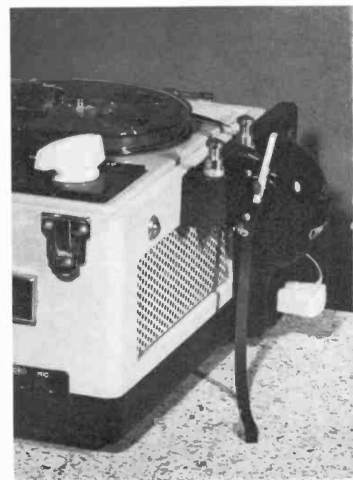
Fig. 2—The shut-off/alarm is fastened semi-permanently to the side of the recorder. To put it into use at any time, just thread the tape around the guide posts before going on to the take-up reel and flip on one or both of the toggle switches. Here the tape has come to the end, releasing its pressure on the white switch actuator, hence stopping the machine.
