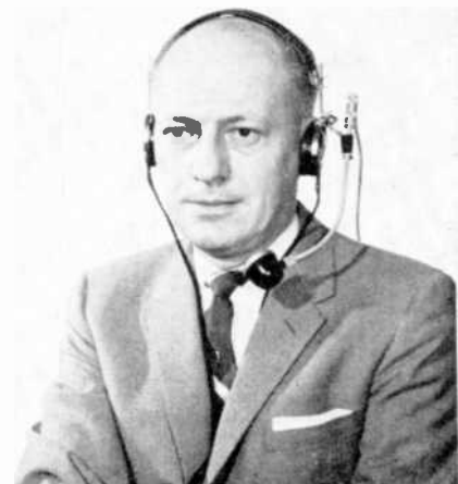
The 260 in use. Note how mike is held clear of face to avoid interference with reading or following text matter.
