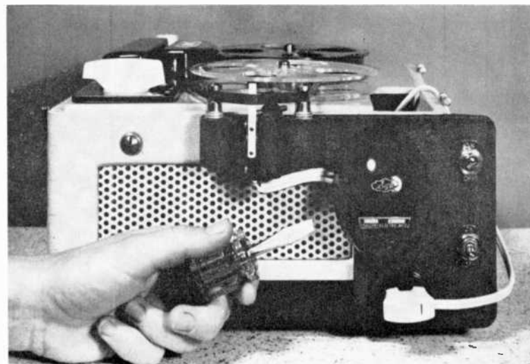
Fig. 7—The completed unit again, fastened to the recorder with three wood screws (also painted). Notice that the white wire and plug coming from the recorder go directly to the amphenol receptacle. And that the plug from the shut-off/alarm—and not from the recorder directly—goes over to a 110-volt AC wall socket. The special "wrinkle" varnish presents a professional appearance.
