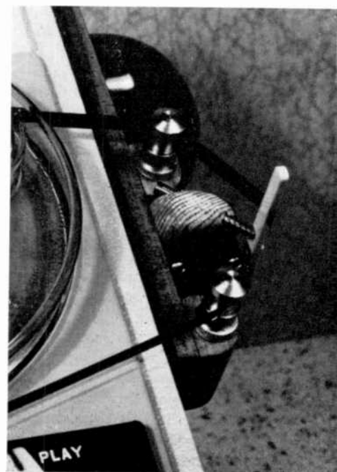
Fig. 5—So that the tape will "ride" easily between the guide posts and over the white switch actuator, it's essential that it be kept exactly upright (at a perfect right angle to the flow of the tape) when pressure is applied by the tape. Here, a set-screw acts as a "stop" and permanently keeps the actuator from going beyond the desired 90° position.
