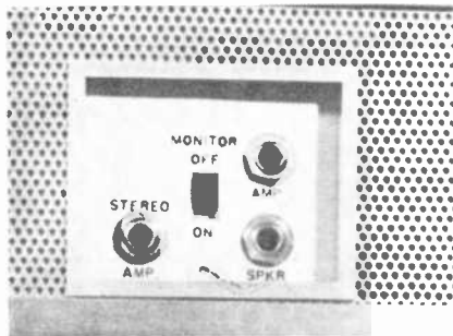
The output panel on the back has jacks for amplifier connection, external speaker and stereo amplifier. The switch permits monitoring while recording.
