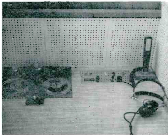
This is a close-up of a typical language laboratory listening booth recently established at Macalester College in St. Paul, Minn. In addition to a two-channel tape deck, the booth includes a control panel, headphones, microphone and provision for the student to talk back and forth with his instructor.
