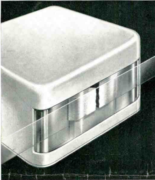
Picture of a recorder head's contact surface, with critical center gap eroded and enlarged by the wearing action of conventional magnetic tape.
