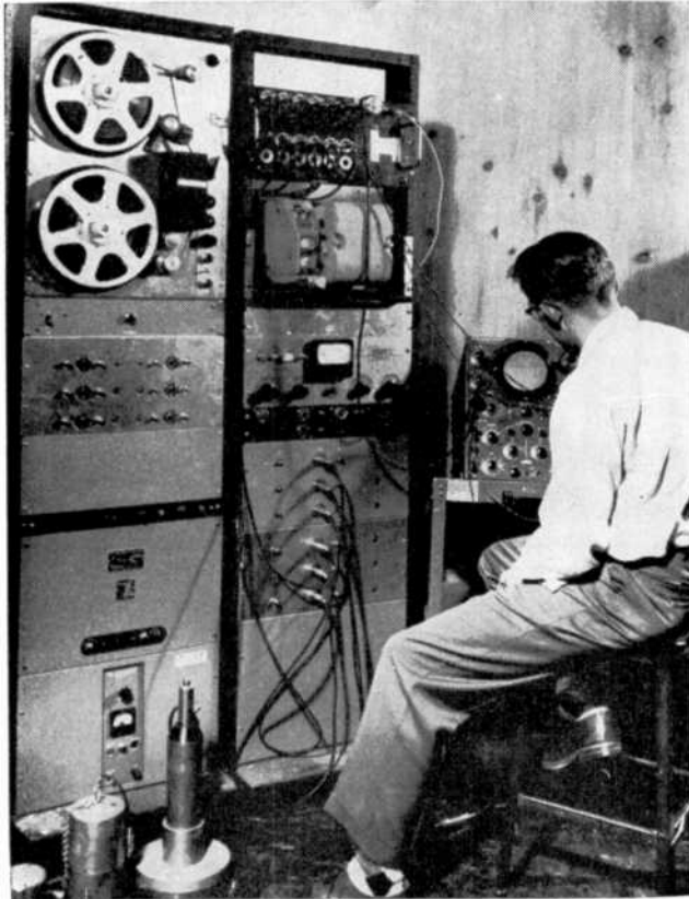
Seismic data such as that involved in earthquake study or in geophysical prospecting for oil is recorded and analyzed on this 7-track Ampex tape unit mounted in a communications type rack.
