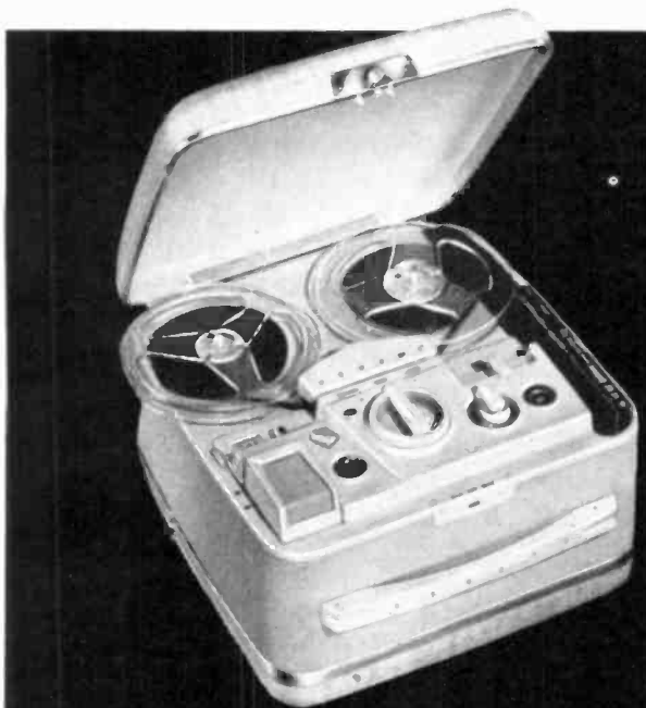
T-1100 DUAL-SPEED CONTEMPORARY. Single knob control, 3-hour play, two matched speakers, 360° sound distribution. FREQUENCY RESPONSE: 3.75 i.p.s. 85-7,000 ± 3DB; 7.5 i.p.s. 75-12,000 ± 3DB. WOW 0.3% Max. With microphone, radio attach. cord, tape, reels, $159.50
