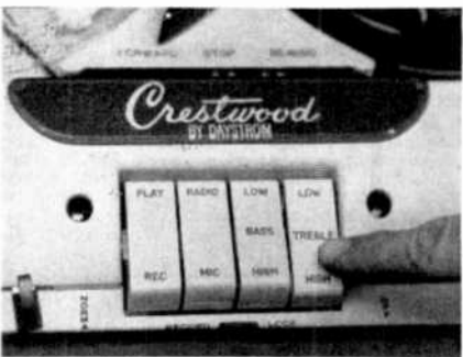
The push button controls are shown here. At the top may be seen the lever which controls the tape motion, forward, rewind and stop. The neon recording level lights are in wells at either side of the push buttons and can be seen clearly in a brightly lighted room.
