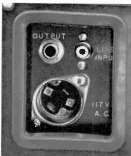
Inputs are located in a recessed well in the end of the case. The line cord and reels are carried in the detachable lid of the unit.
