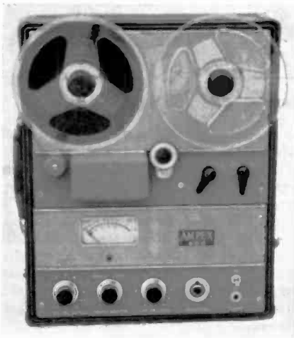
The 600 may be used either vertically or horizontally. Reels are held in place by rubber knobs which grip the drive shafts.
