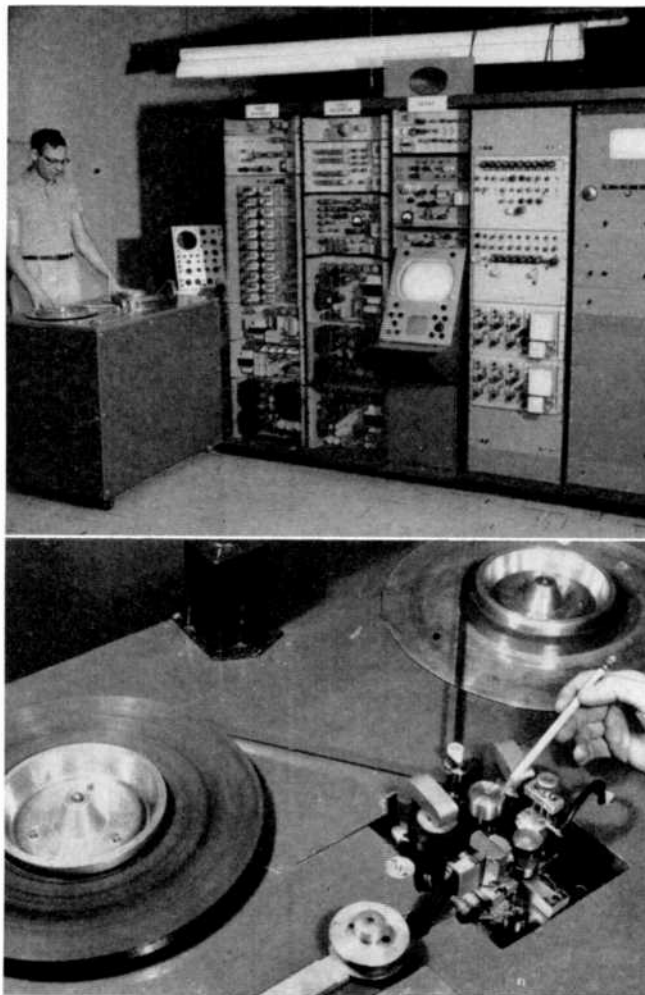
Top: the VTR for recording TV pictures and sound on tape. The complete recording and playback unit will be contained in a cabinet of the approximate size of the one now used for the tape transport alone (at left of picture). Below: the tape drive mechanism for the 12 channel, one-half inch tape running at 100 inches per second.
