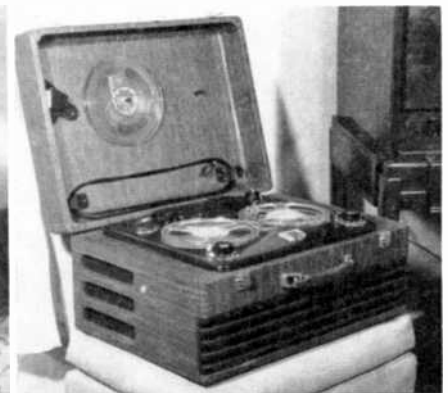
The line and microphone cords are wrapped on cleats in the lid and extra reels of tape are stored on the spring pins.
