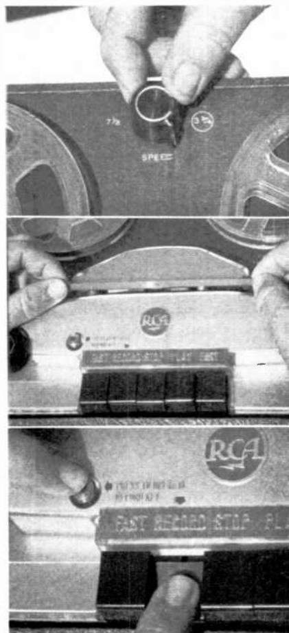
Top: change in speed is effected by turning knob to the desired speed, either 3\frac{3}{4} or 7\frac{1}{2} inches per second. The knob should not be operated while the machine is running. Center: to thread, the tape is dropped in the slot dull side away from the operator. By lightly depressing one of the other buttons, the stop button is released and threading made easier. Lower: to record, both the safety button and the record button must be depressed.
