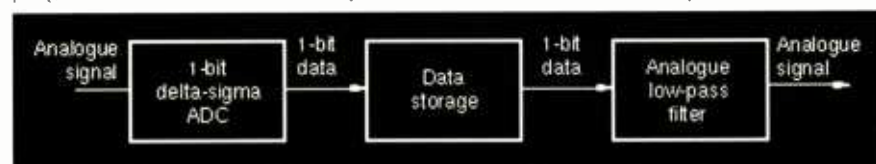
Fig.1: Basic DSD signal chain
