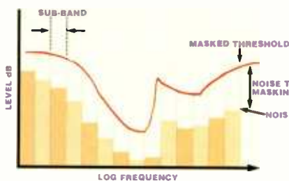
Fig.2c: Sub-band coding mimicking human masking threshold
