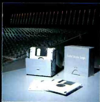
3.5" disk drives allow the use of low cost, high capacity disks for mix data storage
