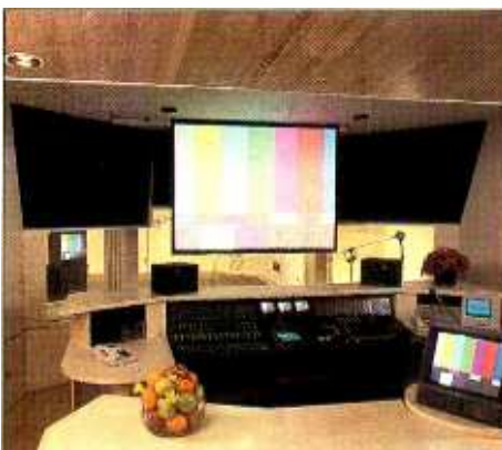
Dual mix-to-picture and sweetening rooms for Editel-Chicago were designed to operate with a central machine room that houses analogue-digital ATRs and a wide selection of video machines
