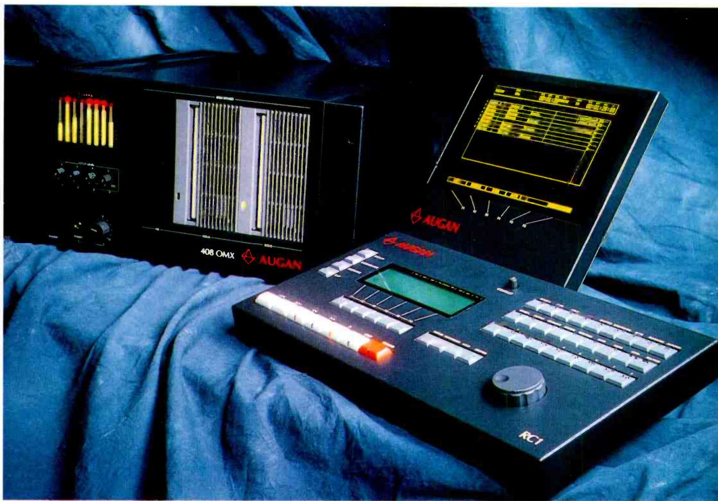
The OMX uses a mixture of optical discs, a hard disk and on-board RAM to provide seamless production
