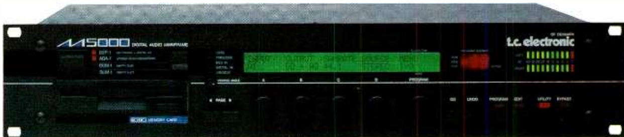
Frequency Response: 10-22KHz, +0,-0.5 dB, Fs=48KHz; THD: < 0.06% 1kHz, 0 dBm; Dynamic Range: >95 dB; Digital Conversion: Linear 18bit 64x in, 20bit 8x out. Max. Level: +22 dBm
