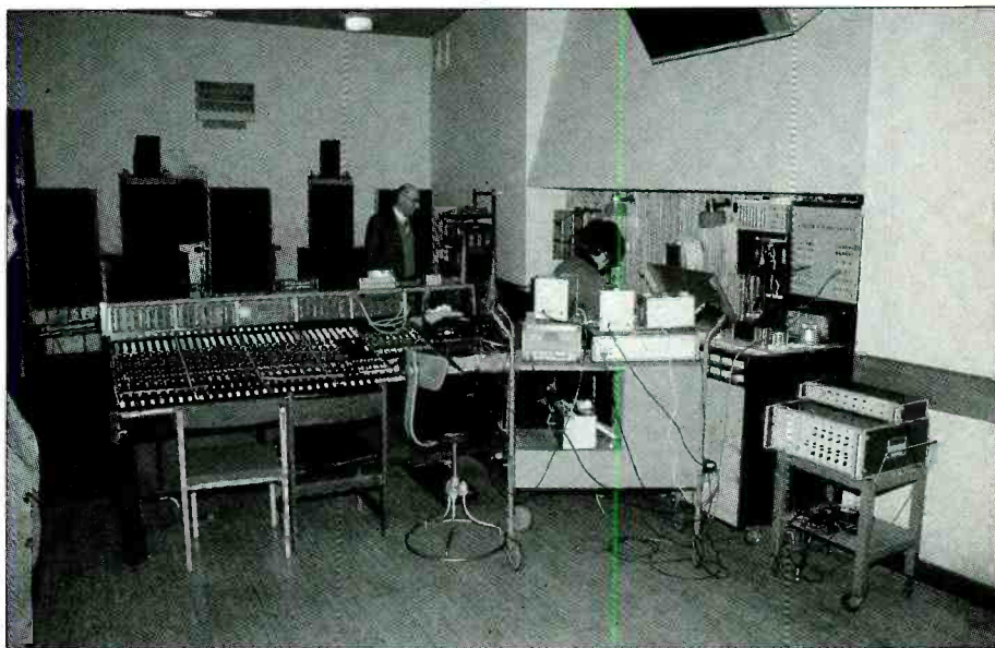
Music control room with Tesla console and Ampex multitrack MM1100 at Lenfilm
