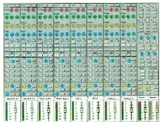
Our AudiMation™ virtual mixer gives you fast, intuitive control over EQ, levels, routing, and other system parameters.
