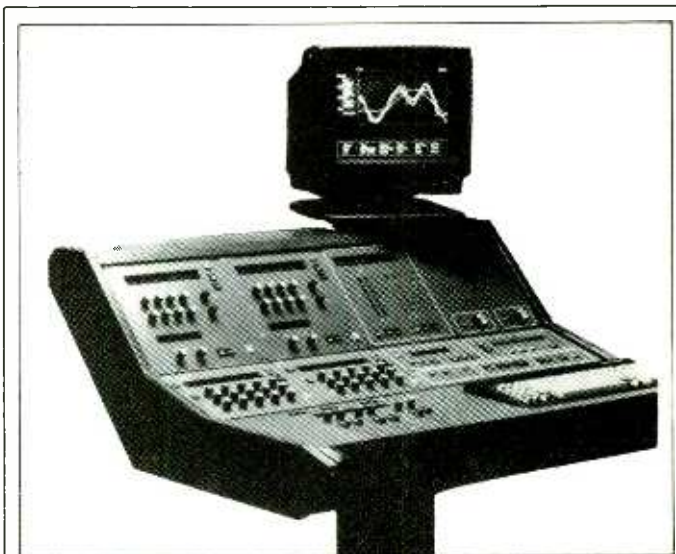
The Muse from Audio Automation is an automated digital console for CD mastering and digital editing. Features include 24 to 56 bit realtime processing, full automation of all parameters and digital inputs and outputs (AES/EBU, SDIF-2, RS-232). Input and output levels are adjusted either via optical pots or 'drawn in' on the high resolution colour monitor. The EQ section is 5-band fully parametric with the dynamics section providing control over ratio, threshold, attack and release settings. The Muse can accept sampling rates of 30 Hz to 100 kHz, thus allowing for future developments.
