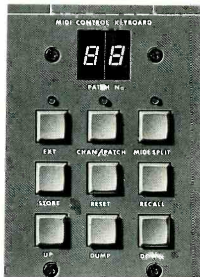
MIDI MUTES CAN BE WRITTEN IN REAL OR STEP TIME, AND RECALLED EITHER INDIVIDUALLY OR AS PATCHES THROUGH THE KEYPAD OR USING A MIDI SEQUENCER
