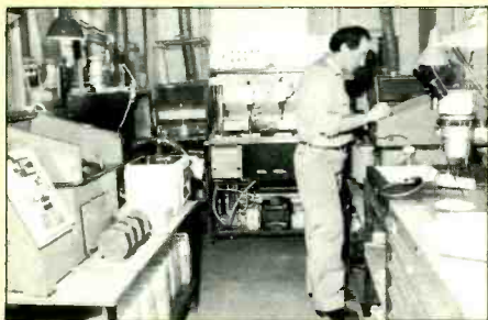
Lapping and final polishing operations on mic housing and backplate
