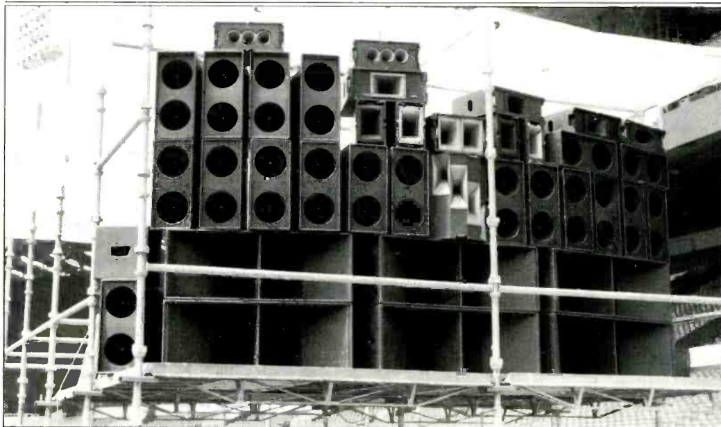
Delay tower placed towards the back of the pitch
