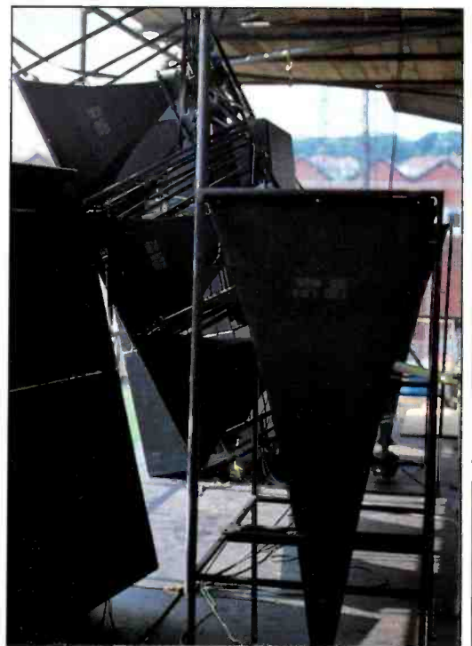
At many venues, houses are very close by. Tilting speakers is one way of reducing sound levels outside the stadium without losing impact within the grounds
