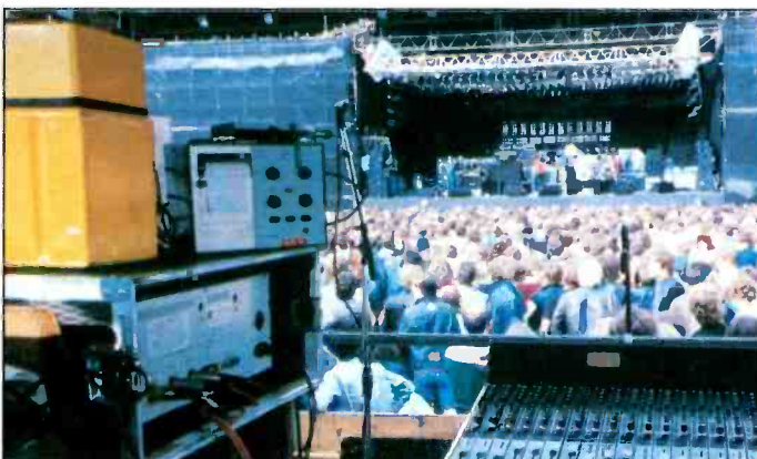
A DOSE meter in action at the Live Aid mixing position
