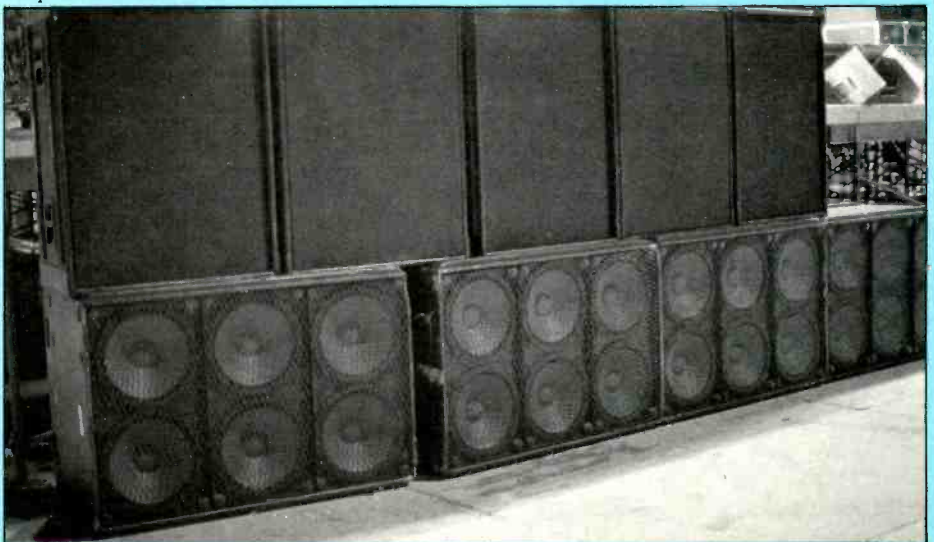
Fig 3: Northwest Sound's bass-augmentation cabinet houses six 15 in loudspeakers in a deep infinite-baffle enclosure
